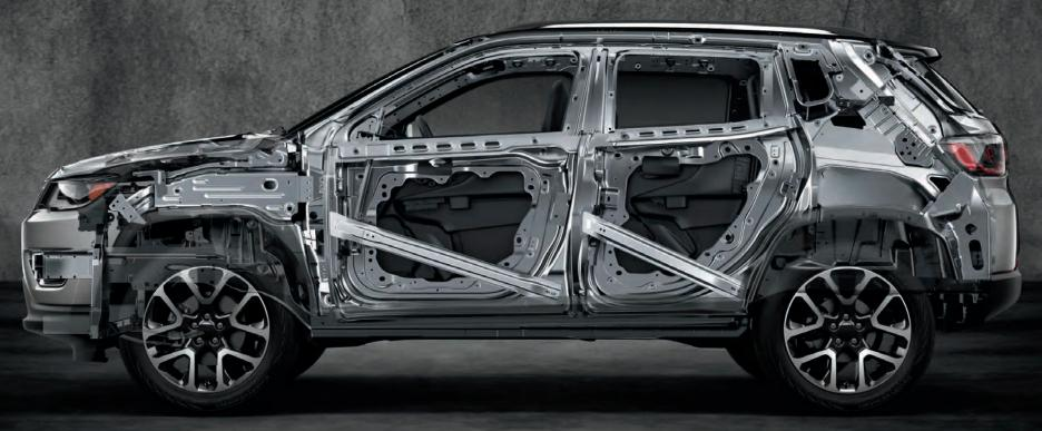
CHASSIS STRENGTH COMPASS DELIVERS EXCEPTIONAL PEACE OF MIND WITH A HERO'S HEART — A STRONG UNIBODY STRUCTURE IS ENGINEERED WITH APPROXIMATELY 70% HOT-STAMPED STEEL. STANDARD.
